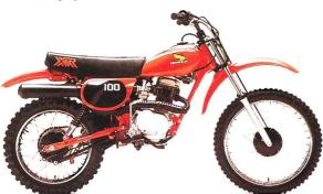
This lightweight dirtbike is easy-to-handle and powered by a forgiving 99 cc OHC four-stroke. Low seat height.
