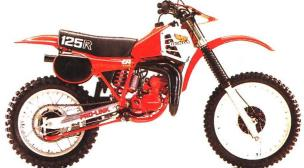
Pro-Link<sup>™</sup> rear suspension and a water-cooled 122 cc reed-valve two-stroke engine make this an all out motocrosser.
