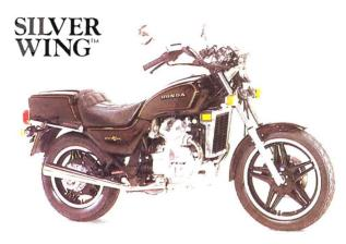
New, mid-sized, shaft driven touring bike with a 497 cc liquid-cooled engine and Pro-Link<sup>rw</sup> rear suspension.
