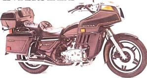
A fully dressed, full-sized touring bike with shaft drive, a 1085 cc liquid-cooled engine and air suspension.
