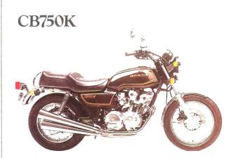
A classic powered by a dependable 749 cc DOHC four-cylinder, four-stroke engine with Pentroof<sup>TM</sup> combustion chamber and four-into-four exhaust. Air-adjustable front forks and halogen headlight.
