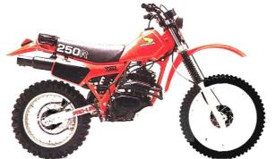
A competition-oriented enduro bike powered by a 249 cc four-stroke engine and equipped with Pro-Link<sup>™</sup> rear suspension. Six-speed gearbox.
