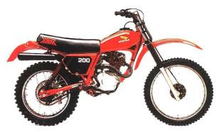
Lightweight, easy-to-ride and fun. This dirtbike is powered by a dependable 195 cc OHC fourstroke engine with six-speed gearbox.
