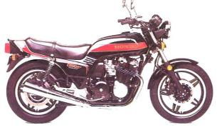
A race-bred total performance motorcycle. 902 cc DOHC four-cylinder engine. Four 32 mm CV carbs. Oil cooler. Needle bearing swing arm pivot. 30-way adjustable shocks with remote reservoir. V-rated tubeless tires.
