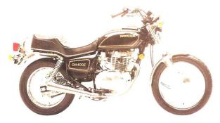
An inexpensive, 395 cc bike featuring a large 3.7 gallon tank. Electric starter, CDI ignition, dual counter-balancers and Power Chamber<sup>™</sup> exhaust system.
