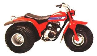
A three-wheeled workhorse with a large frame, a torquey 192 cc OHC four-stroke engine and a five-speed transmission with an automatic clutch.
