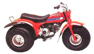
A work or play three-wheeler with a dual-range four-speed gearbox, automatic clutch, large fuel tank and torquey 105 cc four-stroke engine with CDI.
