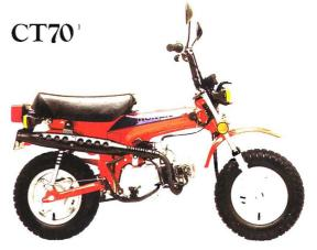
A small, inexpensive street legal trailbike with a 72 cc OHC four-stroke and automatic clutch.
