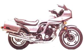
A beautiful state-of-the-art sport motorcycle. 1047 cc six-cylinder, DOHC four-stroke engine with 24 valves. Pro-Link<sup>™</sup> rear suspension. Air forks. Sports fairing, detachable saddlebags.
