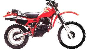
A powerful, new competition-oriented enduro bike with a 498 cc four-stroke engine, reedvalve assisted induction, Pro-Link<sup>TM</sup> rear suspension and a double leading shoe front brake.
