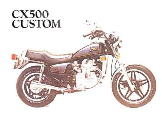
A mid-sized custom bike with shaft drive and a liquid-cooled 497 cc V-twin engine.
