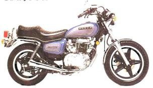
Custom styled, 395 cc twin. Air-adjustable forks. Power Chamber™ exhaust system. Engine counter-balancers.
