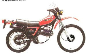
A versatile, dual-purpose bike powered by a 249 cc four-stroke that's powerful, economical and easy-to-maintain.
