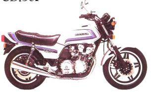
The basis for Team Honda Superbike racers. 749 cc DOHC four-cylinder engine. 16 valves. Air forks. 30-way adjustable shocks.
