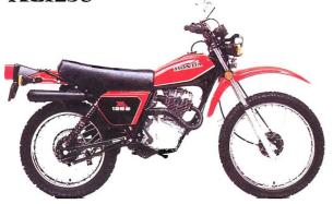
Big bike features on a smaller, economical dual-purpose bike with a 124 cc four-stroke engine and six-speed transmission.
