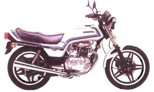
Stylish high performance. Six-valve 395 cc OHC counter-balanced twin, six-speed transmission and Power Chamber<sup>™</sup> exhaust system. Air forks and lightened front disc brake.
