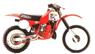
A works type motocrosser with water-cooled 246 cc two-stroke engine and Pro-Link<sup>™</sup> rear suspension.
