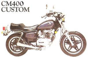
395 cc counter-balanced twin. This new custom features a 3.7 gallon fuel tank and highlighted ComStar<sup>™</sup> wheels.
