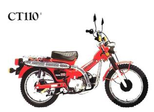
A lightweight, rugged street legal trailbike with dual range gearbox, step through frame and automatic clutch.
