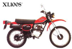
A scaled down dual-purpose bike with an economical 99 cc OHC engine and five-speed transmission.
