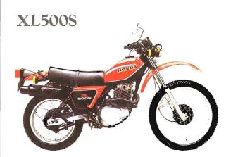
A strong, dual-purpose motorcycle powered by a 498 cc OHC engine mounted in a tough, light frame.
