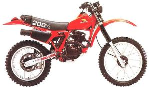
A nimble, very competitive enduro bike with a torquey 195 cc four-stroke engine, six-speed gearbox and Pro-Link<sup>™</sup> suspension.
