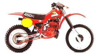
Works type motocrosser with Pro-Link<sup>™</sup> rear suspension and powered by an awesome 431 cc reed-valve two-stroke engine.
