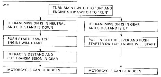
1. Turn the ignition key to "ON" and the engine stop switch to "RUN."
