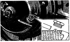
1 Final gear oil 2 Correct oil level
