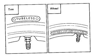
Tube-type Wheel →Tube-type Tires only Tubeless-type Wheel →Tube-type or Tubeless tires
