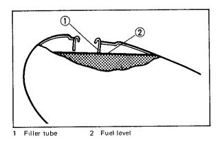
Recommended fuel: Regular gasoline For Australia<sup>-</sup> Unleaded fuel only Fuel tank capacity Total<sup>-</sup> 16.8 L (3.7 Imp gal, 4.4 US gal) Reserve
