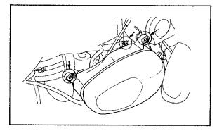
4. Remove the air filter case cover
