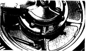
1 Final gear drain plug
