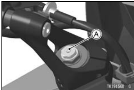
A. Rebound Damping Force Adjuster
