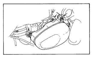
4. Remove the air filter case cover.
