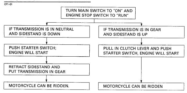
1 Turn the ignition key to "ON" and the engine stop switch to "RUN"
