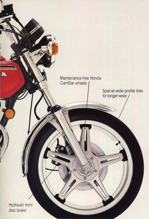
If you've never ridden before, or if you just want to ride "automatically," the new Hawk Hondamatic is made for you. The Hawk Hondamatic™ is the world's first semi-automatic mid-size road bike. No clutch! Put the transmission into "low" range for taking off and low-speed riding. For highway riding or sustained cruising, use "high" range. The Hawk Hondamatic is easy to operate. And first-timers won't look like first-timers either. They'll look like pros.
