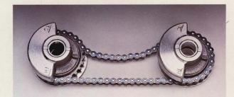
**Vibration Counterbalancers.** To diminish the vibration normally associated with twin-cylinder machines, Honda has equipped the Hawk with a pair of primary-phase counterbalancers (one in front and one behind the crankshaft). They smooth out engine vibration to a level approaching that of many four-cylinder machines for a smoother, more enjoyable ride overall.
