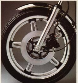
ComStar Wheels. Standard on the Hawk II and Hawk Hondamatic, the Honda ComStar™ wheel is a new concept in motorcycle wheels. It combines the strength of a cast wheel with a small, predetermined amount of flex, like a spoke wheel. The ComStar wheel looks great. And, it's designed for maintenance-free use.
