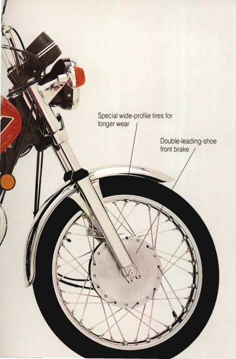
The 1978 Honda Hawk™ series (Type I, Type II and Hondamatic) is a revolutionary new family of motorcycles designed to fulfill the midrange motorcycling needs of riders from expert to beginner. All the Hawks share the same revolutionary high-performance, big-bore, ultra-short-stroke, overhead-cam, three-valve engine technology. And, as you'll see, they also share many other innovative features, but they are still individually distinctive and have their own unique personalities and appeal.
