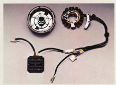
**Tri-Pulser™ CD Ignition.** The Hawk's new Tri-Pulser capacitor discharge ignition is designed to provide high-output, low-maintenance fire power. There are no points to wear out or burn up. The ignition senses the engine rpm and *electronically* sets the timing advance for efficient hot-spark performance.
