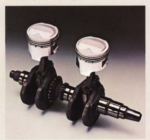
**Big-Bore, Ultra-Short-Stroke.** The Honda Hawk engine combines big-bore pistons (70.5mm) and an ultra-short-stroke crankshaft (50.6mm—about half the length of a king-size cigarette) to provide exceptionally-high rpm potential without excessive piston speed. The result is a high-revving engine able to produce astonishing power.
