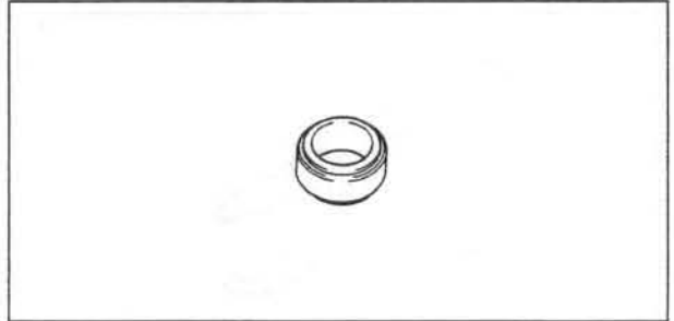
Head Pipe Outer Race Press Shaft: 57001-1075
