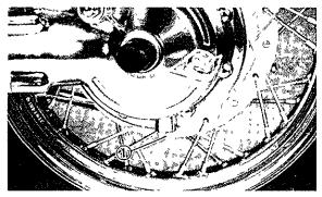
Final gear drain bolt
