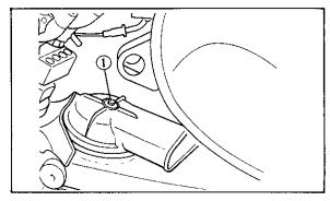
1 Air filter case fitting screw
