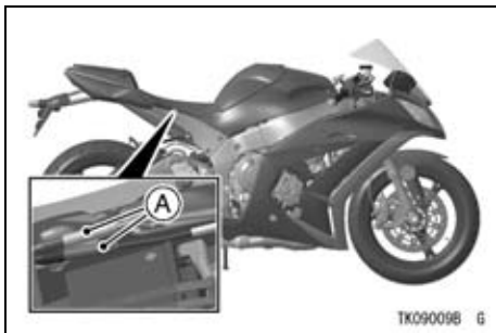
A. Exhaust Device Cables
