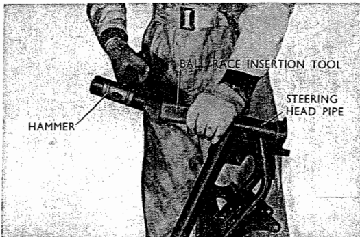
Fig. 4.39 Driving in ball race
