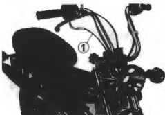
Fig. K4-5 ① Throttle cable
