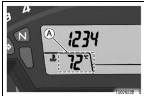
A. Lap Counter/Coolant / Intake Air Temperature Meter
