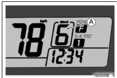
A. Gear Position Indicator (Normal mode)
