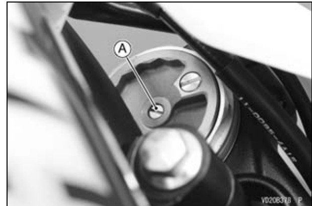
A. Compression Damping Adjuster
