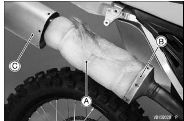
A. Silencer Wool B. Muffler Body C. Muffler Cover
