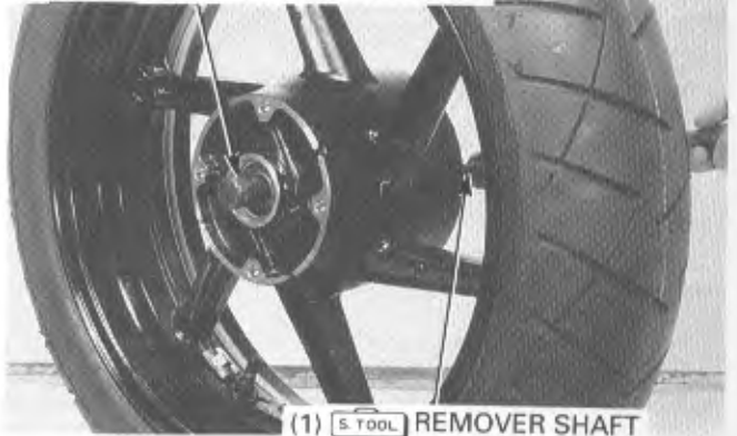
(2) (S TOOL) BEARING REMOVER HEAD
