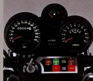
Instruments include a racereliable electric tach, large speedometer, fuel gauge, and resettable tripmeter.
