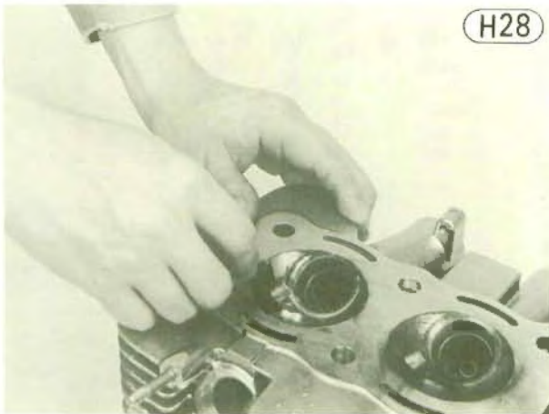
Plastic Plate used for Cylinder Head Volume Measurement
