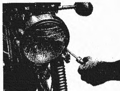
Fig. 54 Adjusting beam horizontally
