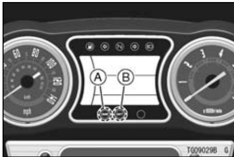
A. Electronic Cruise Control Indicator Light B. Electronic Cruise Control Set Indicator Light
