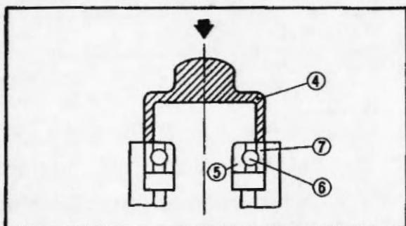
Do not strike the center race ⑤ or balls ⑥ of the bearing. Contact should be made only with the outer race ⑦.
