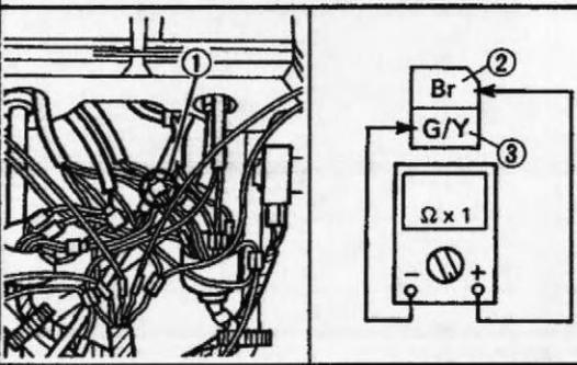
• Check the brake switch for continuity.
