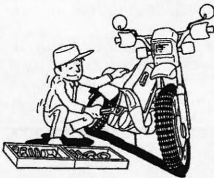
3. When disassembling the machine, keep mated parts together. This includes gears, cylinders, pistons, and other mated parts that have been "mated" through normal wear. Mated parts must be reused as an assembly or replaced.
