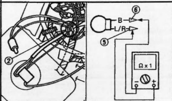
**A** Tail/Brake light bulb socket
