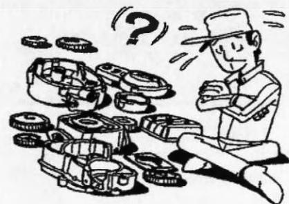
4. During the machines disassembly, clean all parts and place them in trays in the order of disassembly. This will speed up assembly time and help assure that all parts are correctly reinstalled.
