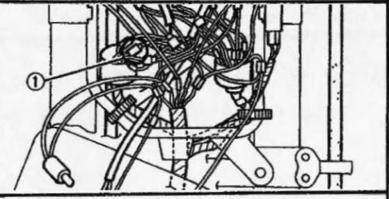
• Connect the Pocket Tester ( $\Omega \times 1$ ) to the handlebar switch (Left) coupler.
