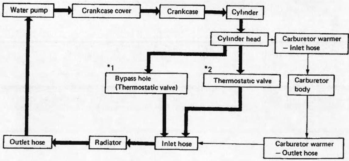
\*1 Coolant is cooled (Less than 65°C (149°F)).
