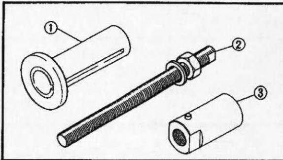
8. Crankshaft Installing Tool
