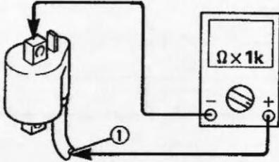
• Measure the Secondary coil resistance.
