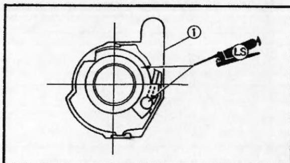
3. Apply the grease to the throttle cable end and cable guide groove at inside of throttle housing ①.
