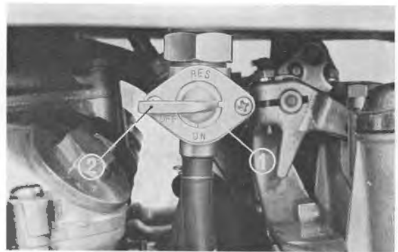
Fig. K1-1 ① Fuel cock ② Lever ③ Fuel cock fixing nut
