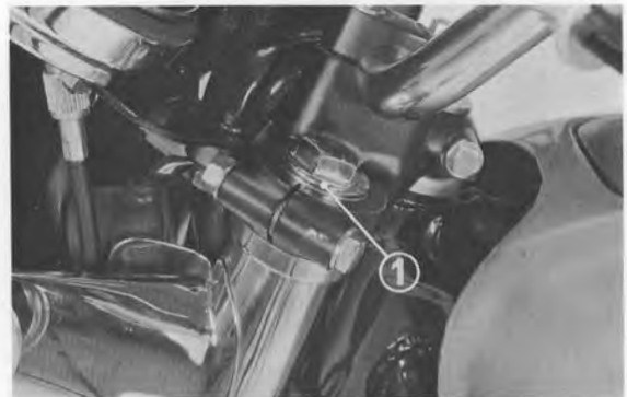
Fig. 2-8 ① Chamfered edge on front fork pipe
