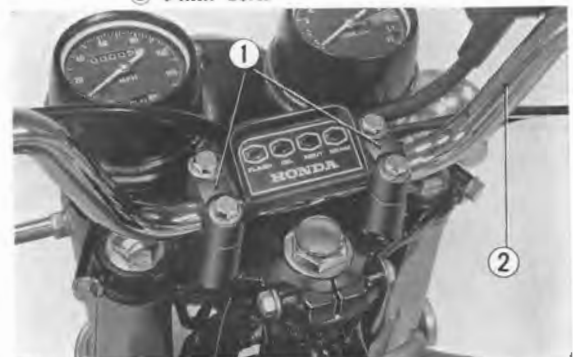
Fig. 239 ① Upper handle bar holders ② Handle bar
