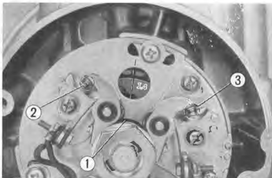
Fig. 13 ① Slipper ③ 2·3 points ② 1·4 points
