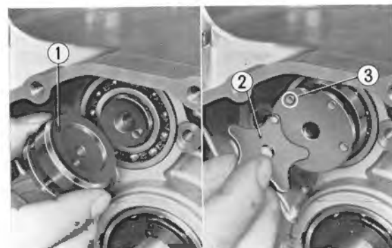
Fig. 372 ① Drum gearshift center ② Drum stop cam plate ③ Lug
