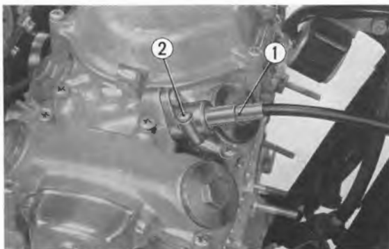
Fig. 44 ① Tachometer cable ② 5 mm screw
