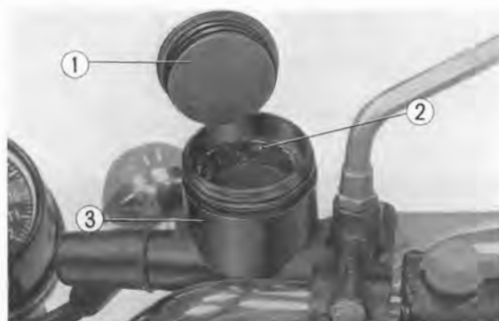
Fig. 223 ① Diaphragm ③ Master cylinder ② Brake fluid
