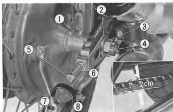
Fig. 38 ① Fork cap bolt ⑤ Adjust bolt ② Mark ⑥ Lock nut ③ Axle nut ⑦ Loosen ④ Cotter pin ⑧ Tighten
