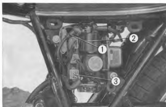
Fig. 48 ① Starting motor cable ② Magnetic switch ③ Wiring coupler
