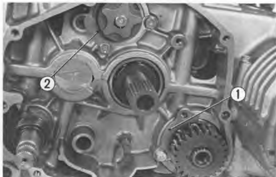
Fig. 364 ① Bearing set plate on primary shaft side ② Bearing set plate on shift drum side
