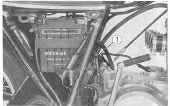
Fig. 53 ① Battery ground cable
