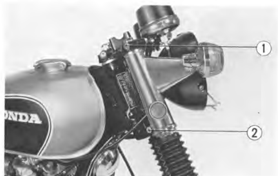
Fig. 253 ① 8 mm setting bolt ② 10 mm setting bolt
