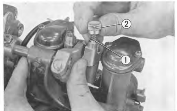
Fig. 192 ① Coil spring B ② Cap nut
