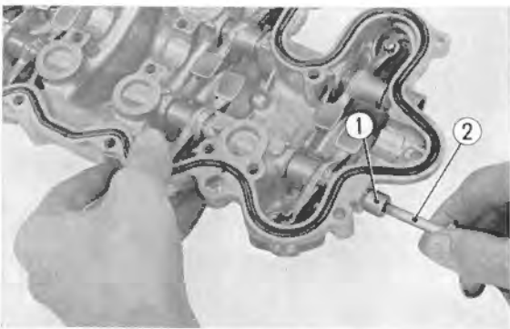
Fig. 66 ① Rocker arm shaft ② 6 mm bolt
