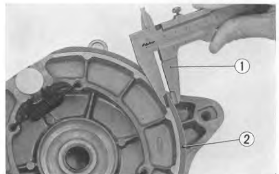
Fig. 230 ① Vernier caliper ② Brake shoe
