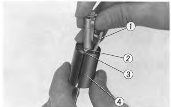
Fig. 185 ① Valve plate ② 3 mm screw ③ Spring washer ④ Throttle valve
