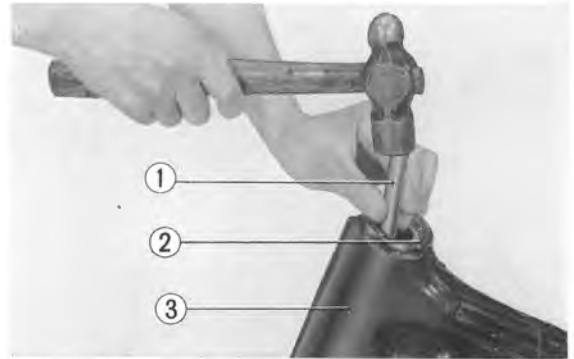
Fig. 265 ① Ball race remover ② Ball race ③ Head pipe
