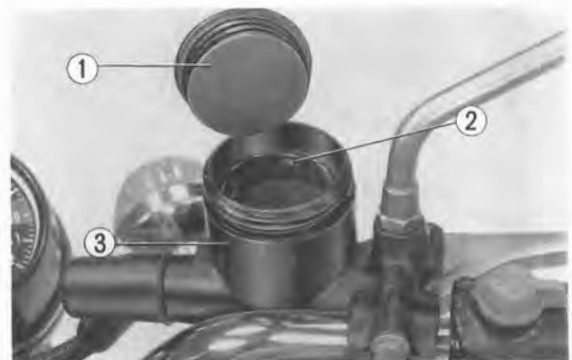
Fig. 32 ① Diaphragm ② Brake fluid ③ Master cylinder
