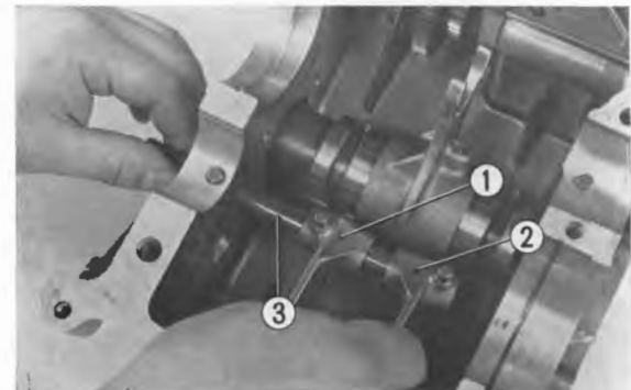
Fig. 369 ① Right gearshift fork ② Left gearshift fork ③ Gearshift fork shaft
