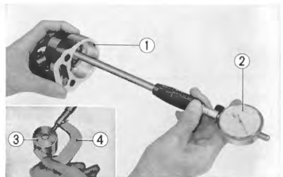
Fig. 217 ① Caliper cylinder ② Cylinder gauge ③ Piston ④ Micrometer
