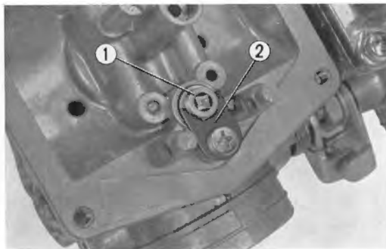
Fig. 182 ① Valve seat ② Clip plate
