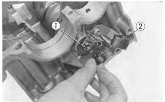
Fig. 130 ① Gear shift drum ② Neutral switch
