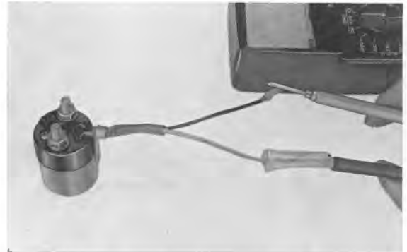
Fig. 304 Primary coil continuity test
