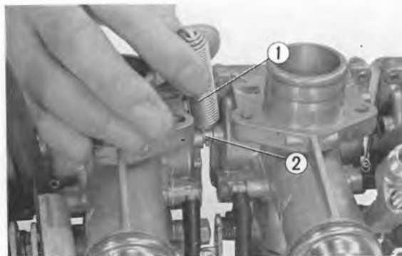
Fig. 190 ① Return spring ② Spring set plate
