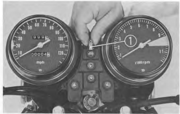
Fig. 2-29 ① Bulb (12V, 3.4W)
