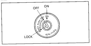
The main switch controls the ignition and lighting systems Its operation is described below.
