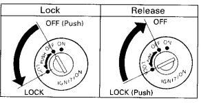
The steering is locked when the main switch is turned to "LOCK" To lock the steering, turn the handlebars all the way to the left. While pushing the key into the main switch, turn it from "OFF" to "LOCK" and remove it. To release the lock, turn the key to "OFF" while pushing.
