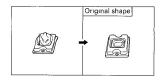
4. The diaphragm will lose its shape from the negative pressure if the brake fluid level goes down too far. Be sure to put the diaphragm back in its original shape before installing it into the master cylinder.
