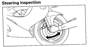
Periodically inspect the condition of the steering. Worn out or loose steering bearings may be dangerous. Place a stand under the engine to raise the front wheel off the ground. Hold the lower end of the front forks and try to move them forward and backward. If any free play can be felt, ask a Yamaha dealer to inspect and adjust the steering. Inspection is easier if the front wheel is removed
