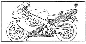
The cowlings indicated in the illustration need to be removed to perform some of the maintenance described in this chapter. Refer to this section each time a cowling has to be removed or reinstalled.
