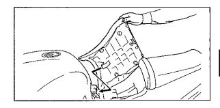
To install the rider seat: Insert the lobe on the front of the seat into the receptacle on the frame. Then push down on the seat.
