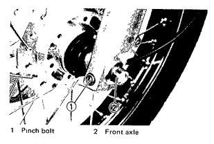
4. Remove the axle and the front wheel Make sure the motorcycle is properly supported.
