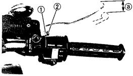
Lock nut 2 Adjuster a  $2 \sim 5$  mm (0.08  $\sim$  0.2 in)
