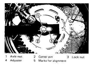
The rear wheel assembly, the collar, the chain adjusters, etc, can be removed from the motorcycle by pulling the wheel axle
