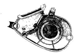
3 Remove the air filter element from its case, and clean it with solvent. After cleaning, remove the remaining solvent by squeezing the element.
