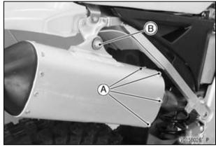
A. Muffler Cover Bolts B. Muffler Mounting Bolt
