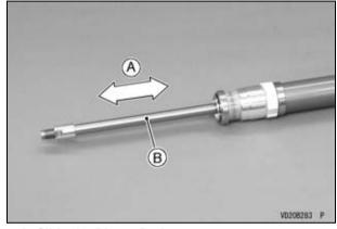
A. Slide the Piston Rod. B. Piston Rod
