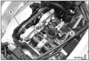
A. Head Cover Gasket B. Spark Plug Hole Gasket
