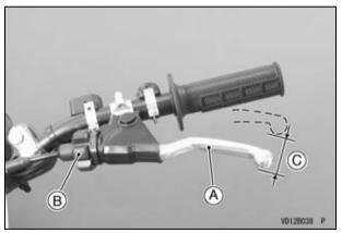
A. Clutch Lever B. Adjuster C. 8 ~ 13 mm (0.3 ~ 0.5 in.)
