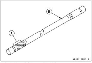
A. Apply molybdenum disulfide grease. B. Oil Passage Hole
