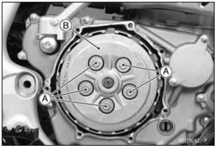
A. Clutch Spring Bolts B. Clutch Pressure Plate • Remove the adjusting washer, needle bearing, push rod holder and push rod.
