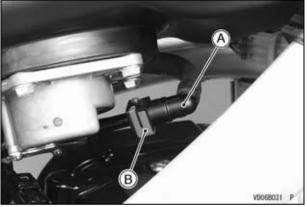
A. Fuel Hose Joint B. Joint Lock
