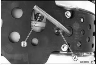
A. Drain Bolt (M6) B. Drain Bolt (M10)
