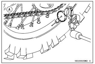
A. Axial Rim Runout Measurement
