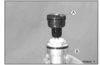
A. Base Valve Assembly B. Cylinder Unit
