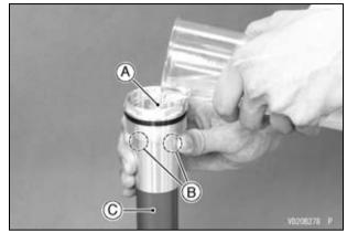
A. Fork Oil B. Oil Holes C. Cylinder Unit
