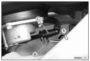
A. Turn B. Joint Lock C. Fuel Hose Joint
