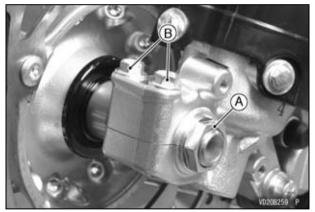
A. Front Axle Nut B. Left Front Axle Clamp Bolts (Loosen)
