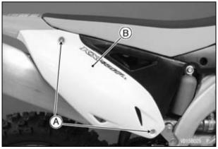
• Remove the muffler cover bolts.
