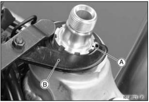
A. Steering Stem Nut B. Stem Nut Wrench (Special Tool: 57001-1100)
