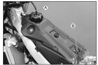
A. Fuel Tank Mounting Bolt B. Band
