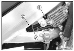
A. Throttle Cables B. Fuel Tank C. Bottom of the Frame (Right Side) • Temporarily tighten the radiator shroud bolts following the tightening sequence.
