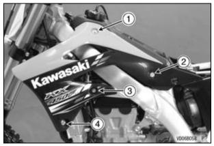
• Tighten the radiator shroud bolts.
