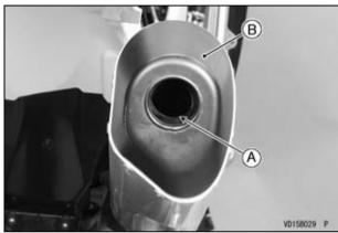
A. Muffler Body End B. Baffle
