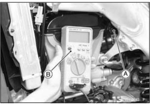
A. Idle Adjusting Screw/Choke Knob B. Tester
