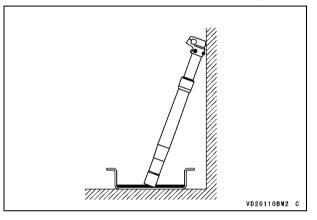
• Clean the threads of cylinder unit and base valve assembly.
