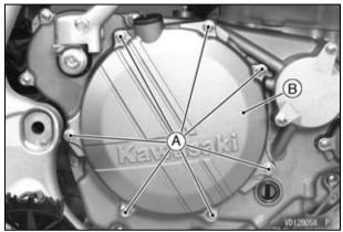
A. Clutch Cover Bolts B. Clutch Cover
