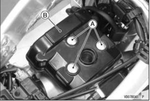
A. Cylinder Head Cover Bolts and Washers B. Cylinder Head Cover • Remove the head cover gasket and spark plug hole gasket.
