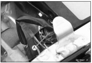
A. Intake Air Temperature Sensor Connector
