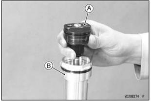
A. Base Valve Assembly B. Cylinder Unit
