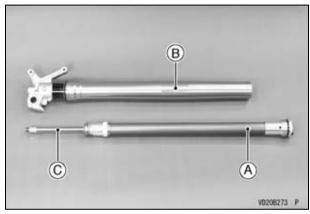
A. Cylinder Unit B. Outer Tube C. Piston Rod
