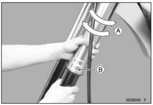
A. Pull down by twisting. B. Front Fork • Using the top plug wrench, 49 mm (special tool: 57001-1653), remove the fork top plug from the outer tube and slowly slide down the outer tube.
