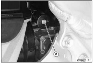
A. Idle Adjusting Screw/Choke Knob
