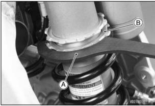
A. Hook Wrench (Special Tool: 57001-1101) B. Spring Preload Adjusting Nut
