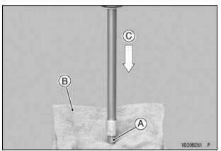
A. Piston Rod End B. Heavy Cloth C. Pump the Piston.
