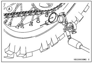
A. Radial Rim Runout Measurement
