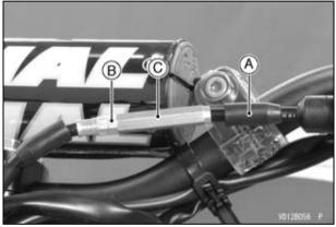
A. Dust Cover B. Locknut C. Adjusting Nut • Tighten the locknut.
