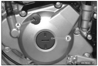
A. Timing Inspection Cap B. Flywheel Nut Cap • Bring the piston to the Top Dead Center (TDC) of its compression stroke to inspect the valve clearance (the position at the end of the compression stroke) by aligning the top mark with the groove on the magneto cover while turning the crankshaft counterclockwise.
