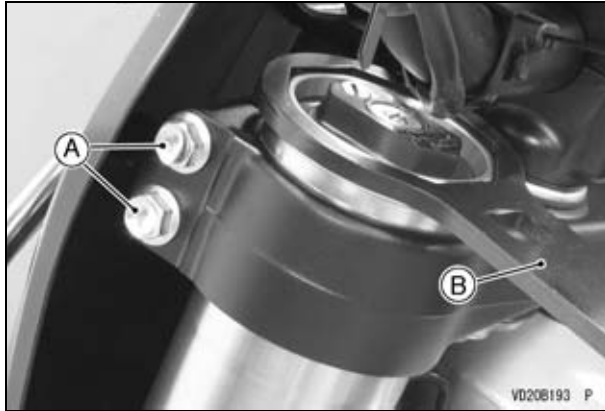
A. Front Fork Clamp Bolts (Upper) B. Top Plug Wrench (Special Tool: 57001-1645)
