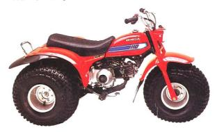
A work or play three-wheeler with a dual-range four-speed gearbox, automatic clutch, large fuel tank and torquey 105 cc four-stroke engine with CDI.
