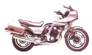
A beautiful state-of-the-art sport motorcycle. 1047 cc six-cylinder, DOHC four-stroke engine with 24 valves. Pro-Link™ rear suspension. Air forks. Sports fairing, detachable saddlebags.
