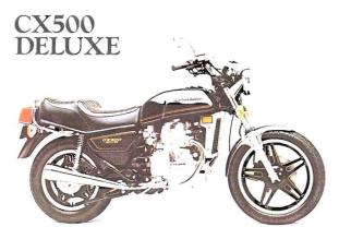
Shaft drive, and a liquid-cooled 497 cc V-twin engine make this motorcycle quiet, comfortable and easy-to-maintain. Air forks. Halogen headlight.
