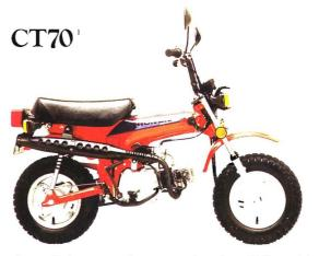
A small, inexpensive street legal trailbike with a 72 cc OHC four-stroke and automatic clutch.
