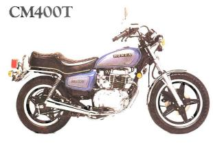
Custom styled, 395 cc twin. Air-adjustable forks. Power Chamber<sup>TM</sup> exhaust system. Engine counter-balancers.
