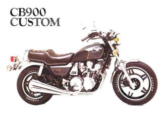
A 902 cc DOHC four-cylinder custom. Honda's exclusive Select-Range  $^{\text{TM}}$  dual ratio sub-transmission and shaft drive.
