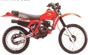
A nimble, very competitive enduro bike with a torquey 195 cc four-stroke engine, six-speed gearbox and Pro-Link<sup>TM</sup> suspension.
