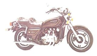
A smooth riding, shaft-driven touring machine with a liquid-cooled, 1085 cc engine and air suspension.
