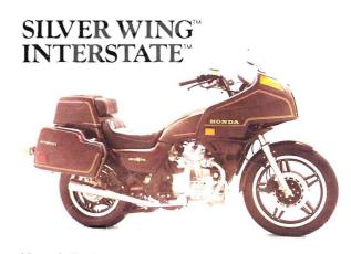
New, fully dressed, liquid-cooled mid-sized touring machine with shaft drive and Pro-Link  $^{\rm TM}$  rear suspension.
