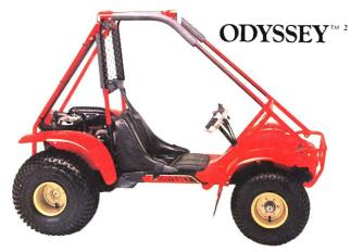
Soft riding flotation tires, two-ply carcass type in the rear, fullcage roll bar and a torquey 248 cc two-stroke engine make this machine a funmobile.
