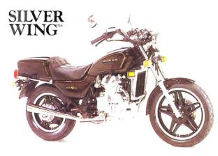
New, mid-sized, shaft driven touring bike with a 497 cc liquid-cooled engine and Pro-Link ru rear suspension.
