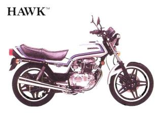
Stylish high performance. Six-valve 395 cc OHC counter-balanced twin, six-speed transmission and Power Chamber<sup>TM</sup> exhaust system. Air forks and lightened front disc brake.
