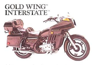
A fully dressed, full-sized touring bike with shaft drive, a 1085 cc liquid-cooled engine and air suspension.
