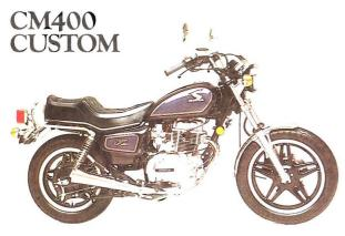
395 cc counter-balanced twin. This new custom features a 3.7 gallon fuel tank and highlighted ComStar $^{TM}$  wheels.
