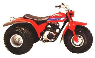
A three-wheeled workhorse with a large frame, a torquey 192 cc OHC four-stroke engine and a five-speed transmission with an automatic clutch.
