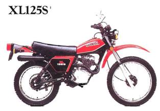
Big bike features on a smaller, economical dual-purpose bike with a 124 cc four-stroke engine and six-speed transmission.
