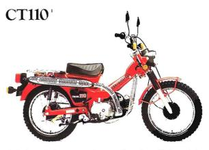
A lightweight, rugged street legal trailbike with dual range gearbox, step through frame and automatic clutch.
