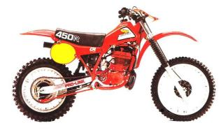
Works type motocrosser with Pro-Link™ rear suspension and powered by an awesome 431 cc reed-valve two-stroke engine.
