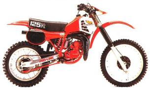
Pro-Link<sup>™</sup> rear suspension and a water-cooled 122 cc reed-valve two-stroke engine make this an all out motocrosser.
