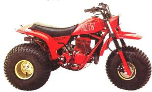
Three-wheeled sports spectacular. Full suspension and a 248 cc reed-valve two-stroke engine.
