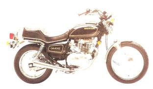
An inexpensive, 395 cc bike featuring a large 3.7 gallon tank. Electric starter, CDI ignition, dual counter-balancers and Power Chamber<sup>TM</sup> exhaust system.
