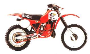
A works type motocrosser with water-cooled 246 cc two-stroke engine and Pro-Link™ rear suspension.
