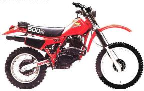
A powerful, new competition-oriented enduro bike with a 498 cc four-stroke engine, reed-valve assisted induction, Pro-Link<sup>TM</sup> rear suspension and a double leading shoe front brake.
