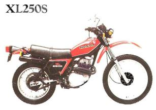
A versatile, dual-purpose bike powered by a 249 cc four-stroke that's powerful, economical and easy-to-maintain.
