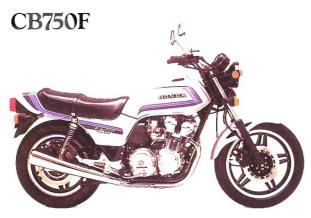
The basis for Team Honda Superbike racers. 749 cc DOHC four-cylinder engine. 16 valves. Air forks. 30-way adjustable shocks.
