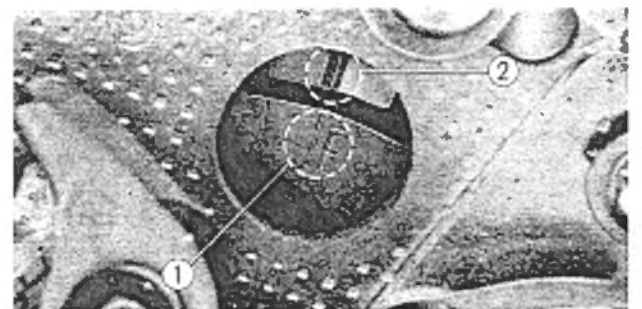
Fig. 2-6 ① Mark "F" 1.4 ② Matching mark
