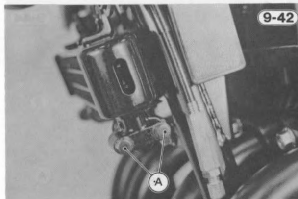
A. 0.80 kg-m (69 in-lbs) of Torque
